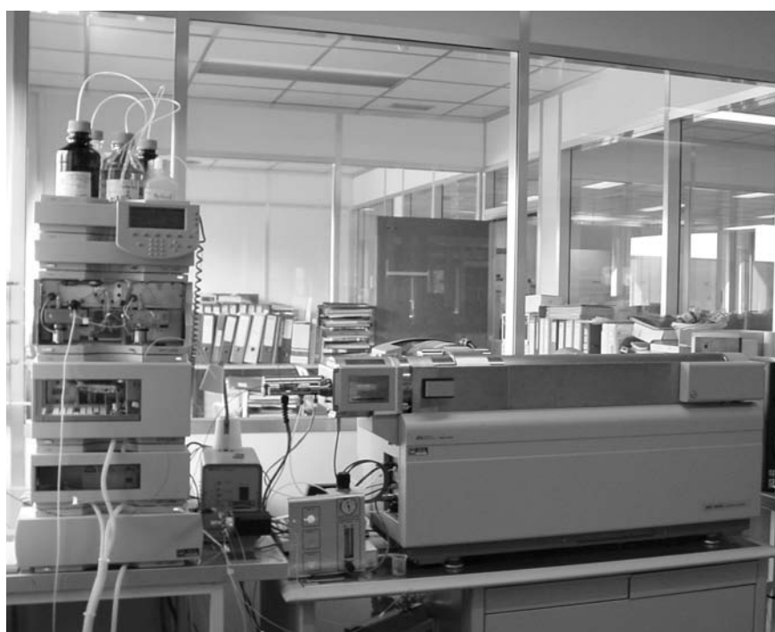
Liquid chromatography - tandem mass spectrometry system (LC-MSMS). Photograph taken at Laboratoire Pasteur Cerba.
