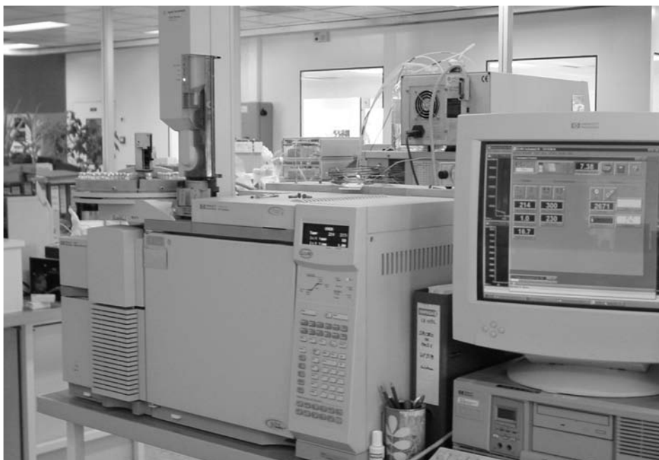
Gas chromatography - mass spectrometry (GC-MS) system Photograph taken at Laboratoire Pasteur Cerba
