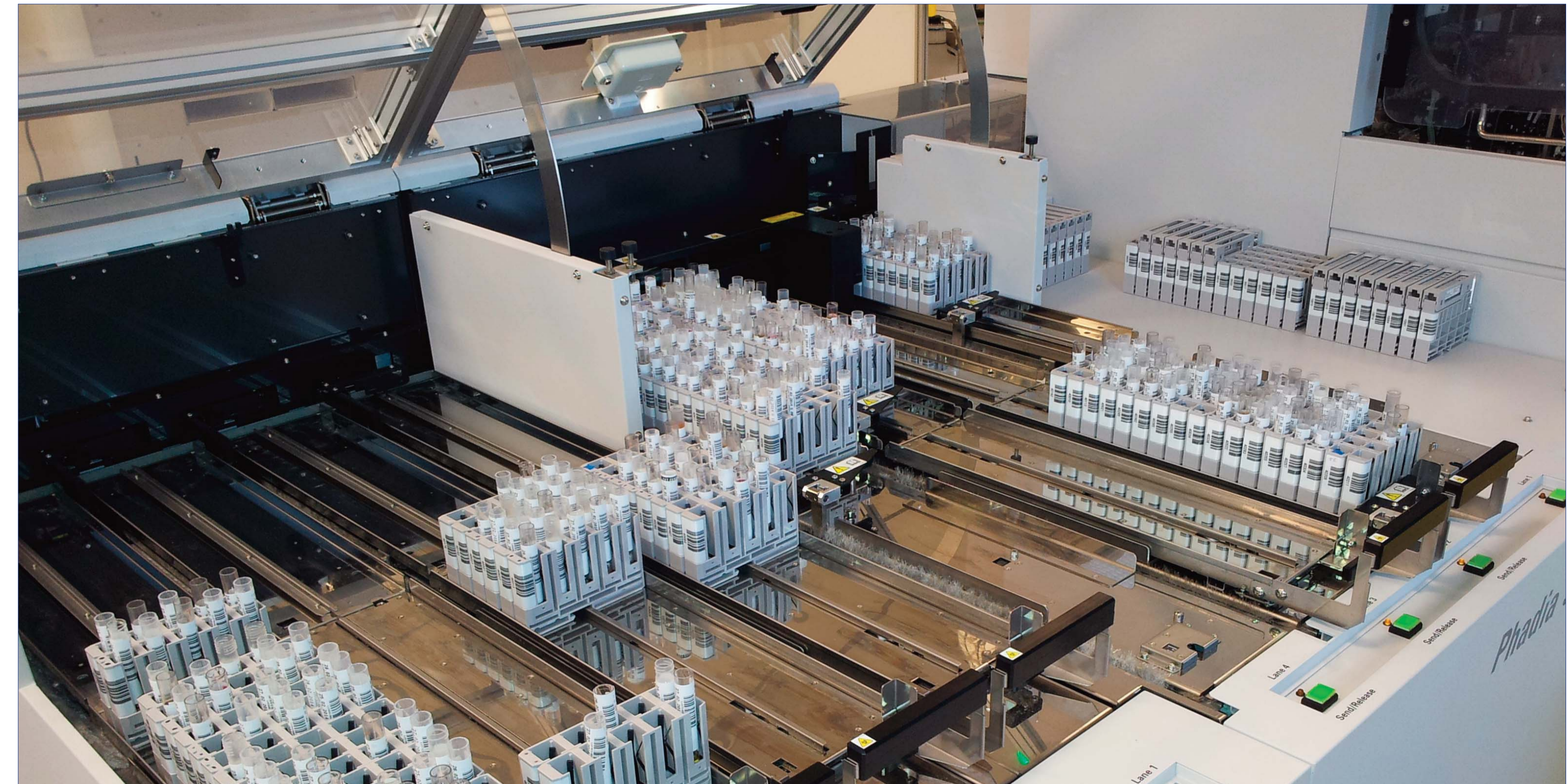
Rack Input/Output module (160 racks) Loading area for samples, IQC, ImmunoCAP/EIA wells, Calibrators/CC.
